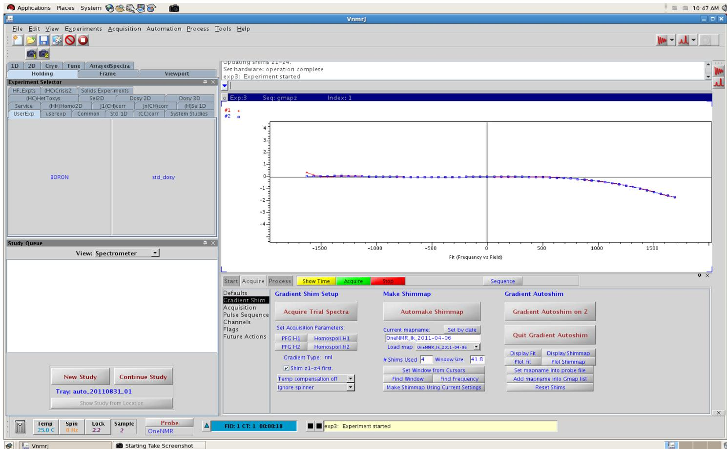
Representative good lineshape from test sample: less than 5 Hz wide at 0.55%, less than 8 Hz wide at 0.11%
