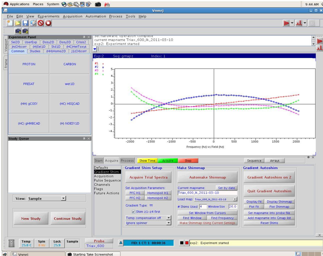
First field map from full length sample starting from default shims—in this case, mostly  $z^3$  and  $z^4$  error, very little  $z^1$  or  $z^2$ . Gradient shimming easily handles this.
